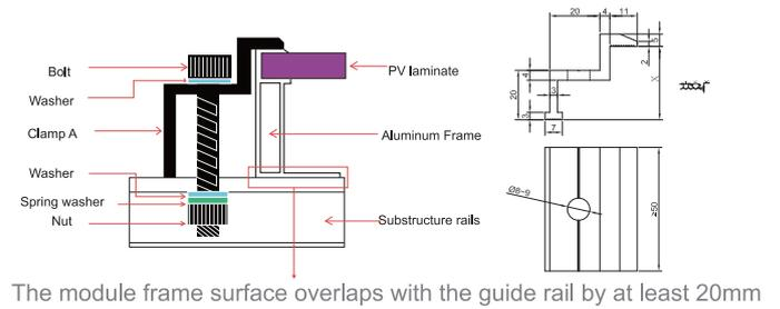
Clamp A The clamp used on the sided module
