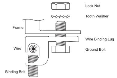
Figure 6: Installation methods
